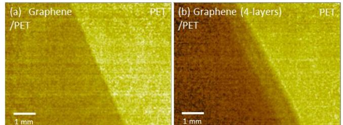
**Fig. 3.** Transmission THz images of (a) single-layer graphene and (b) 4-layer graphene on the PET sheet after image compensation.
