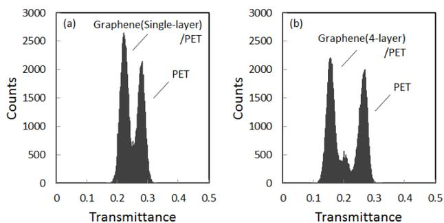
**Fig. 4.** Histogram of transmittance for (a) single-layer graphene and (b) 4-layer graphene on the PET sheet, obtained at 4.28 THz.
