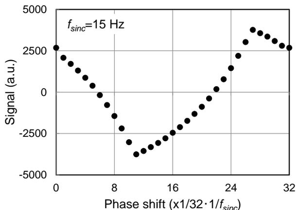
**Fig. 5.** Phase dependence of camera signal, using the phase shifter at synchronization frequency of 15 Hz.
