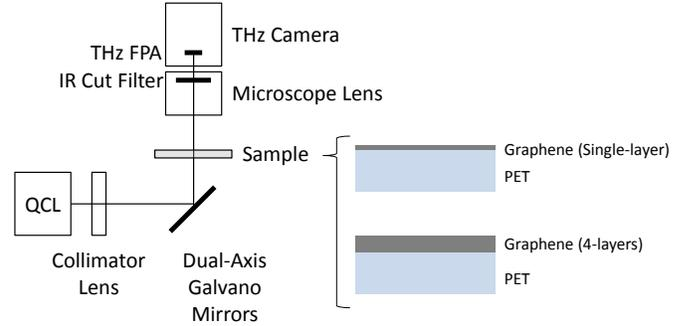
**Fig. 1.** Schematic diagram of the experimental setup for transmission THz imaging.
