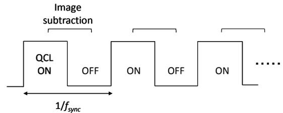
**Fig. 2.** Explanation of lock-in imaging when QCL is used as THz source.
