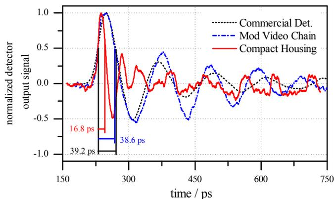
**Fig. 3:** Normalized detector output signal obtained by a 30 GHz sampling oscilloscope. The compact Housing increases the video bandwidth by more than a factor of two and at the same time reduces the ringing of the signal significantly.
