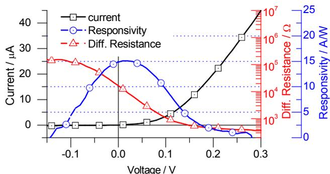
Fig. 2: IV characteristic for the compact detector module. It has a differential resistance of about 16 k $\Omega$  and a current responsivity of about 14.8 A/W at Zero-Bias.
